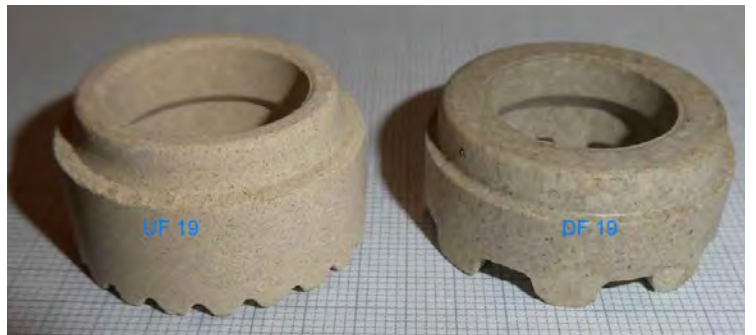
Fig. 11 • Ceramic ferrule for direct welding on the left and for through-deck stud welding on the right.
